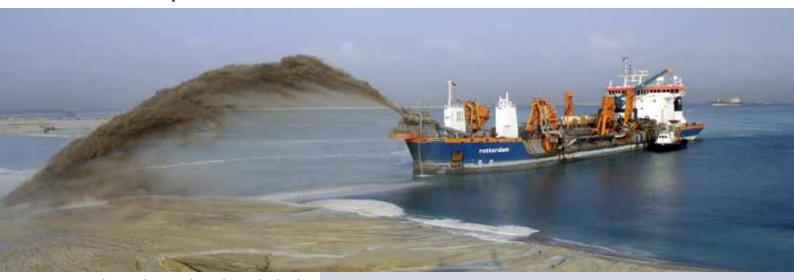
Sand-nourishment along the Netherlands coast: a flexible answer to coastal erosion, a viable protection measure, now and for the future with uncertainties about the rate of accelerated sea level rise, and in the meantime sand nourishment schemes increase the resilience of the coastal zone. (photo: Van Oord)
