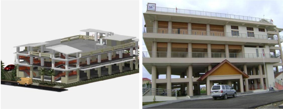
Figure 5: *Sea Defence Consultancy design for escape building (left), and constructed escape building in Banda Aceh (right). (source: SDC- Sea Defence Consultancy Project)*
